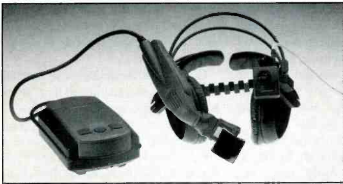
Figure 2. This wearable computer system allows a service technician to carry needed information with him, or to use the internet to obtain it.
